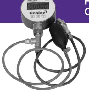
Tinsley Flow Meter Calibrators are portable, easy-to-use kits for verification of the accuracy of Differential Pressure instruments, Recorders, Controllers, Transmitters and Indicators. The differential pressure design incorporated enables calibration of flowmeters.
