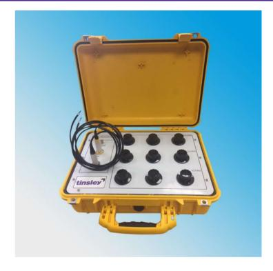
Designed for the checking and calibration of insulation testers at voltages of up to 5000V DC, the Tinsley Model 4720 high resistance decade boxes provides up to 9 decades of resolution.
